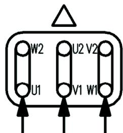
**Connection diagram for three-phase motors**
